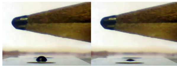
338 Fig. 9. Picture of a prototype Braille dot at rest (left) and when a voltage is applied (right). A video of the dot in action is available at
