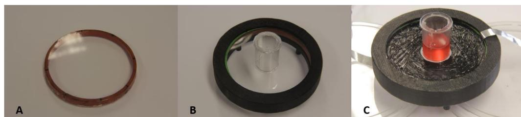
**Figure 4:** The bioreactor at various stages of fabrication: A) the membrane, B) the flexible central well, C) the complete bioreactor mounted within its case, containing the cultured cells and 1 mL of medium within the well and equipped with the carbon grease electrodes.
