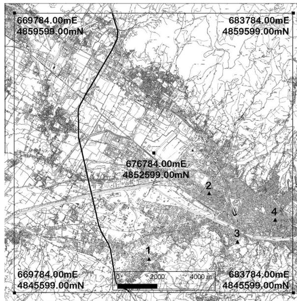
**Fig. 5.** Simulation domain centered at the south edge of the present runway 05 of the Amerigo Vespucci airport. The black triangles labelled with number 1, 2, 3, 4, 5 are the locations of the monitoring. The A1 highway is emphasized with a bold line on the left.
