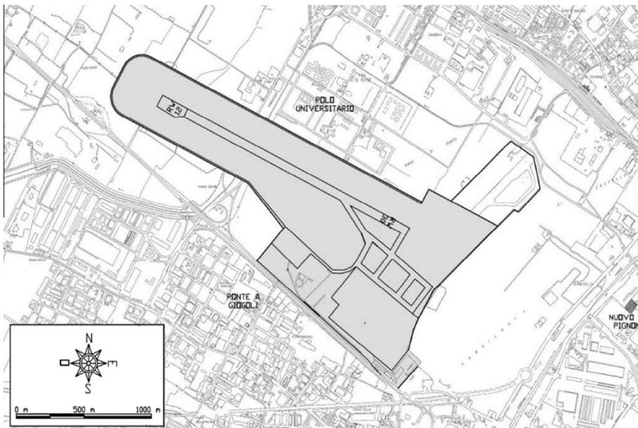
**Fig. 2.** Future layout of the Amerigo Vespucci airport. The direction of the runway is approximately orthogonal to the present one, allowing for different flight trajectories.
