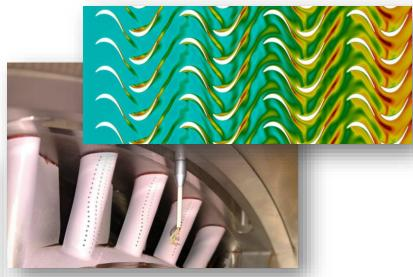
.... to aerothermal characterization of blades and vanes for gas turbines
